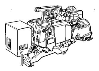
When removing the AC Adaptor/Charger, disconnect the 4-pin cable and remove the AC Adaptor/Charger by sliding it up while pressing the Release Button.
