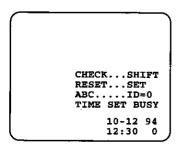
**CAUTION:** Release the Check Button (25) after pressing the Auto White/Auto Black Set Switch (6) to the AWC position. If the Check Button is kept pressed, the camera will not be shifted to the time setting mode.
