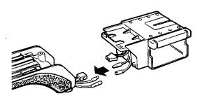
3-3 Attach the Battery Mount Adaptor to the camera by tightening two screws.
