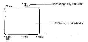
When this button is pressed once more, the recorder is set to the Pause mode (Recording Pause), and the Recording/Tally Indicator and Tally Light will go off.
