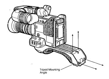
**Note:** When mounting the MII, format VTR AU-45H on this camera, fix the Tripod Mounting Angle in the reverse position onto the Shoulder Pad.
