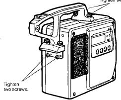
4-2 Mount the VTR to the camera by engaging the connectors and lock mechanism.
