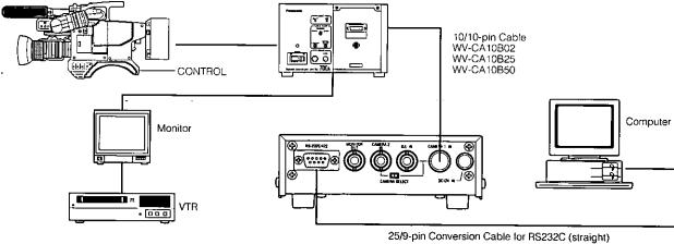
Connect the WV-CA10B02, WV-CA10B25 or WV-CA10B50 10/10-pin conversion cable between the Camera 1 Input Connector on this unit and the Remote Control Box Connector on the Remote Control Unit.
