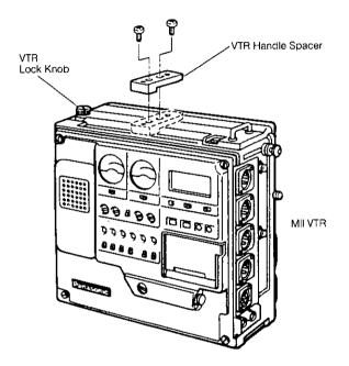
5-2 Mount the VTR to the camera by engaging the connectors and lock mechanism. Tighten the VTR Lock Knob on the VTR and the VTR Handle Fixing screws. Make sure the VTR is securely fixed on the camera.
