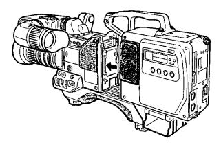
4-3 Tighten the VTR Lock Knobs on the VTR Handle firmly and make sure the VTR is securely fixed to the camera.
