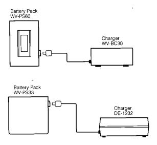
Note: In order to prolong the service life of the Battery Pack, when using the Charger, charge the battery for approximately 15 hours. However, do not charge for more than 24 hours as this will quickly wear out the Battery Pack.
