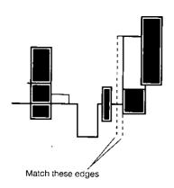
The horizontal phase of the camera can be roughly adjusted by observing the split color bar picture of the program monitor after all switches and controls have been correctly set. Adjust the Horizontal Phase so that the edges of the color bar of the camera and Special Effects Generator roughly match each other.
