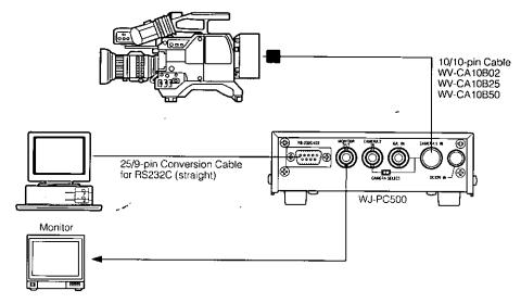
Connect the WV-CA10B02, WV-CA10B25 or WV-CA10B50 10/10-pin cable between the Remote Control Box Connector (37) on this camera and Camera 1 Input Connector on the WJ-PC500.
