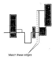
The horizontal phase of the camera can be roughly adjusted by observing the split color bar picture on the program monitor after all switches and controls have been correctly set. Adjust the Horizontal Phase Control for Gen-lock (138) or (198) so that the edges of the color bar of the camera and Special Effects Generator roughly match each other.
