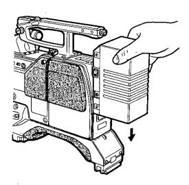
2. Connect the battery cord to the battery connector.
