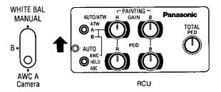
Aim the camera at a white object e.q., white paper or a white wall, within the range of the white balance as shown in the following and make sure that at least 10% or the viewfinder screen is occupied by the white image.
