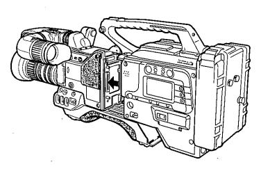
3-3 Tighten two VTR Mounting Screws on the VTR Handle firmly and make sure the VTR is securely fixed to the camera.
