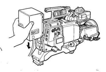
Connect the 4-pin cable to the 4-pin external DC input connector on the cameara.
