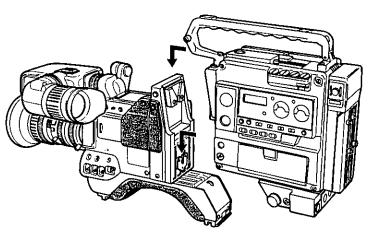
4-2 Secure the VTR with two screws which come with the VTR.
